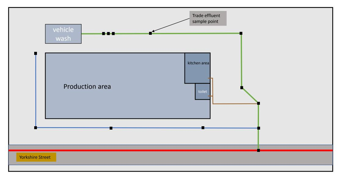
Example of a plan to be used with form G/02 when applying for a trade effluent consent or variation to an existing consent/direction
