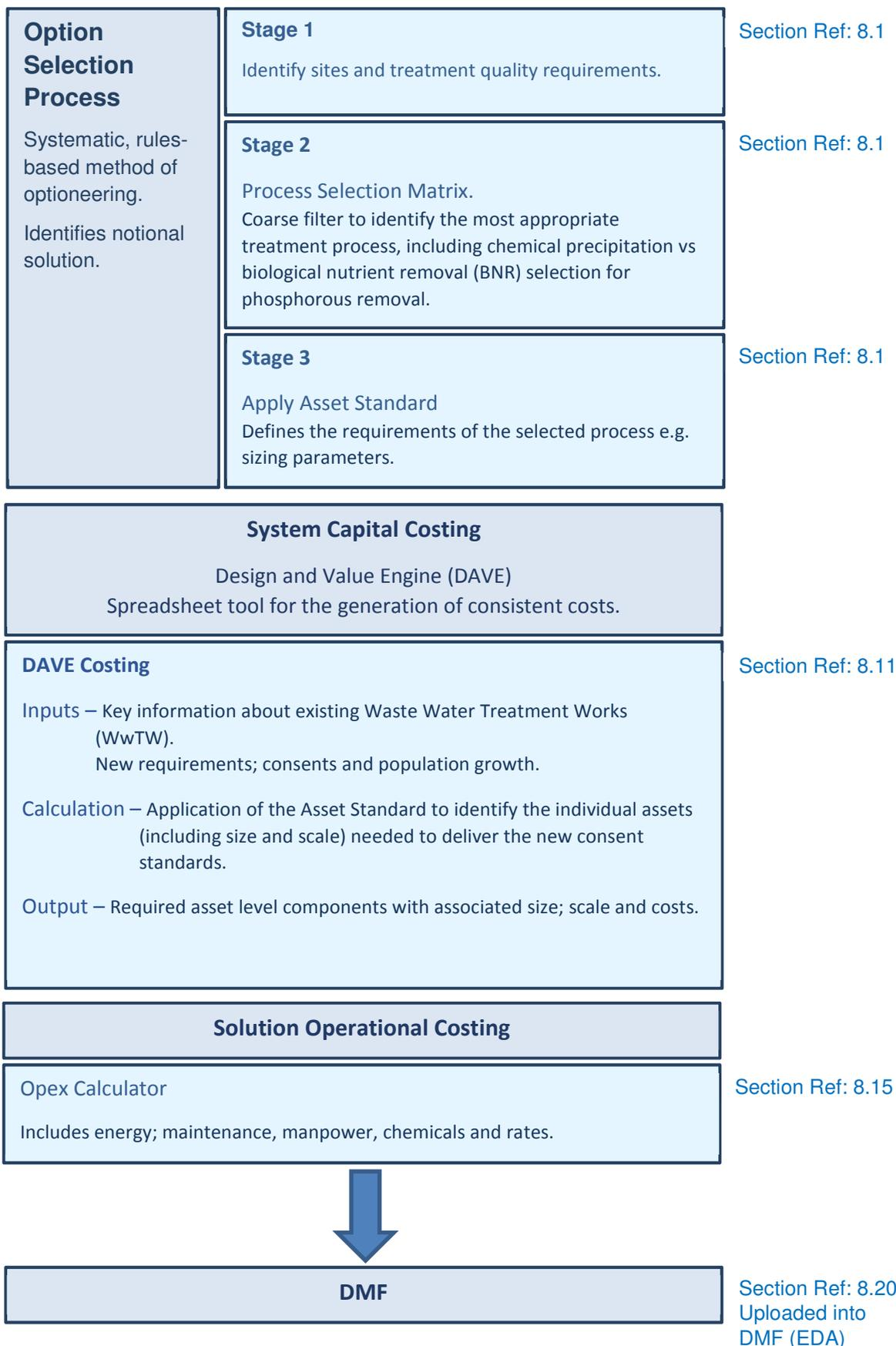
Figure 8.1: The Approach to Waste Water Treatment Costing
