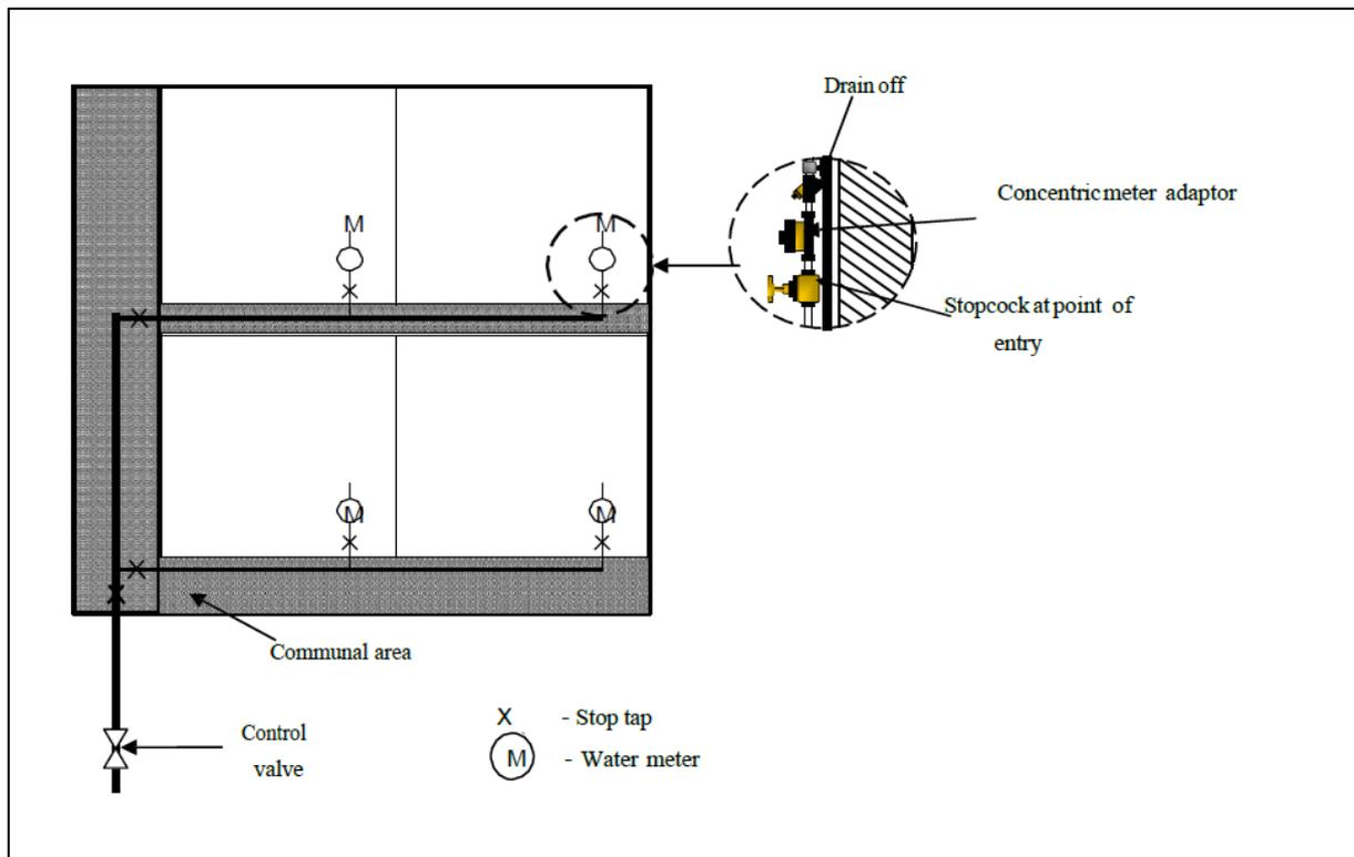
**Figure 63: Standard Drawing (HM.013) Multi Occupancy Building - internal riser with internal meters in each residence**
