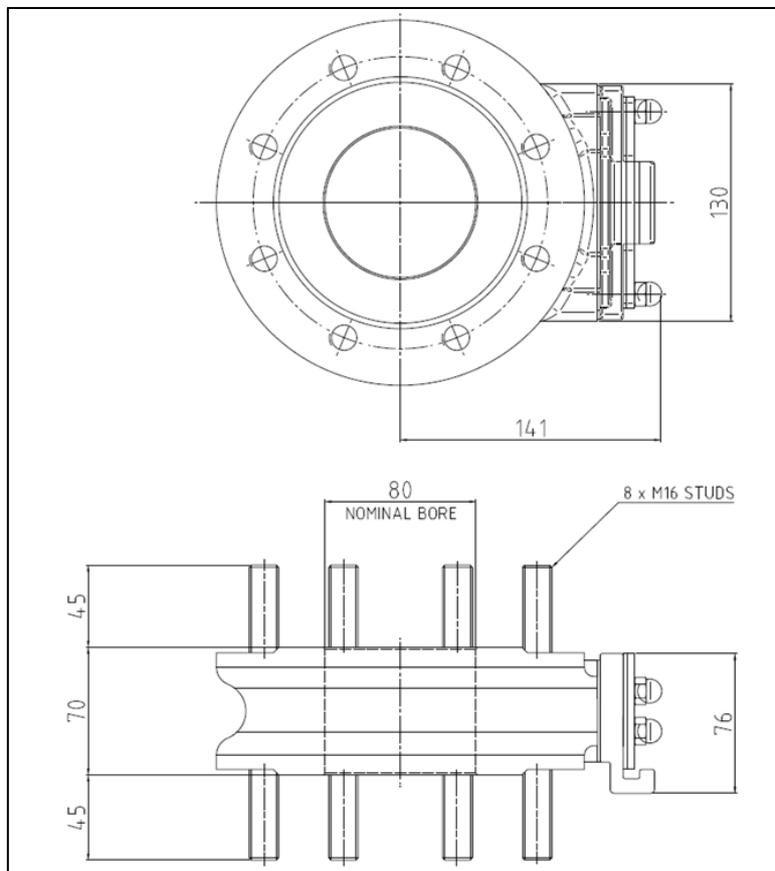
**Figure 41: Standard Drawing (WO.003) MK3 Sandwich Valve**
