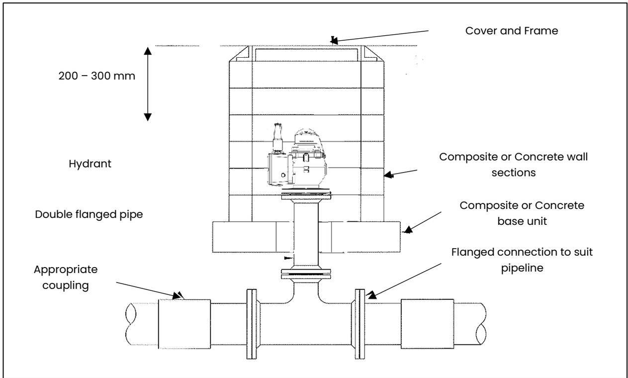
**Figure 40: Standard Drawing (WO.002) Hydrant without Sandwich Valve**
