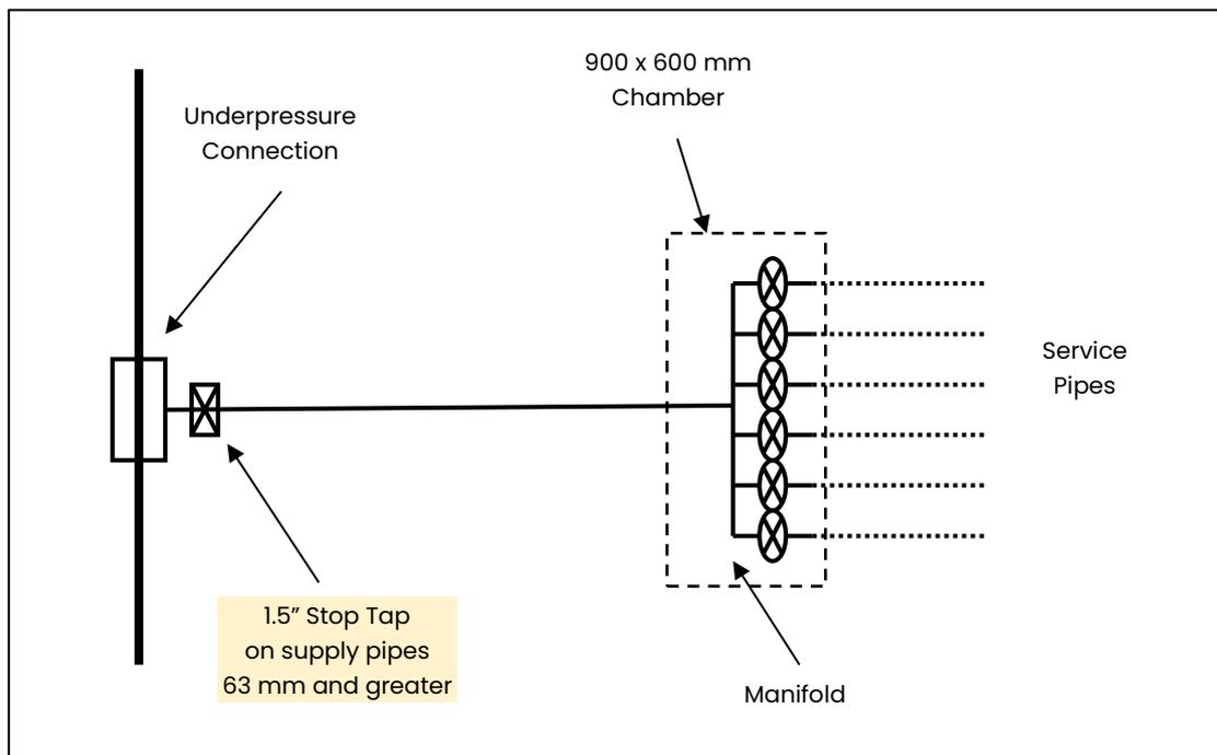
**Figure 25: Standard Drawing (SP.002) Standard Installation Drawing for Manifolds**
