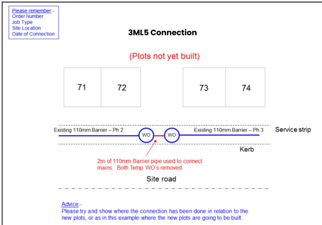
**Figure 17: Example 'As Built' Drawing – 3ML5 Connection**
