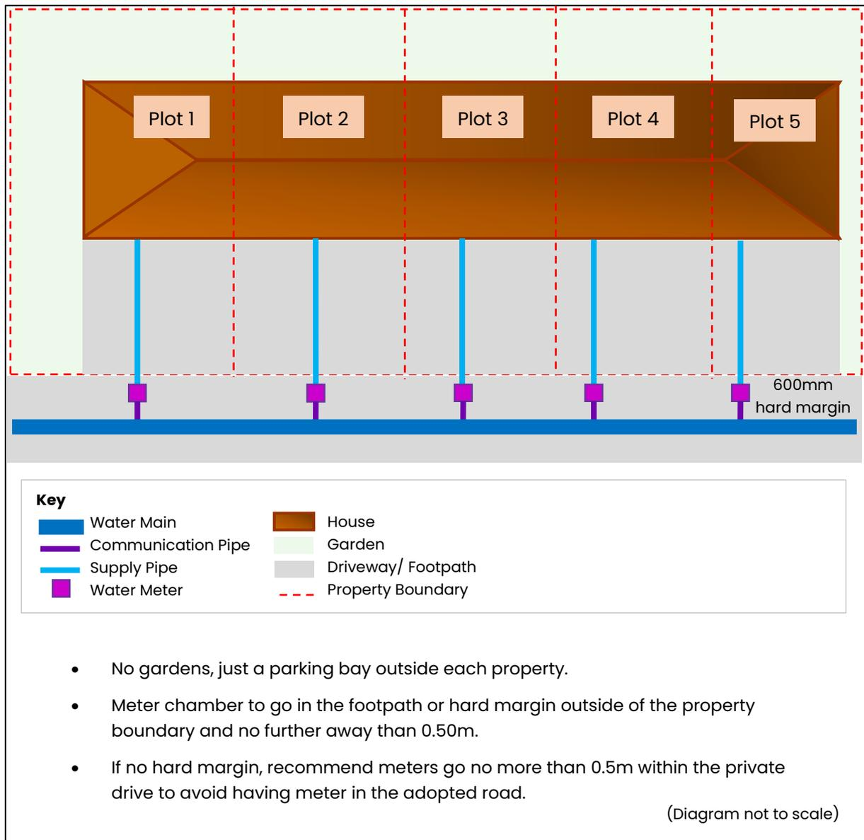
**Figure 31: Standard Drawing (SP.008) Routing and Positioning of Service Pipes – No Front Garden**
