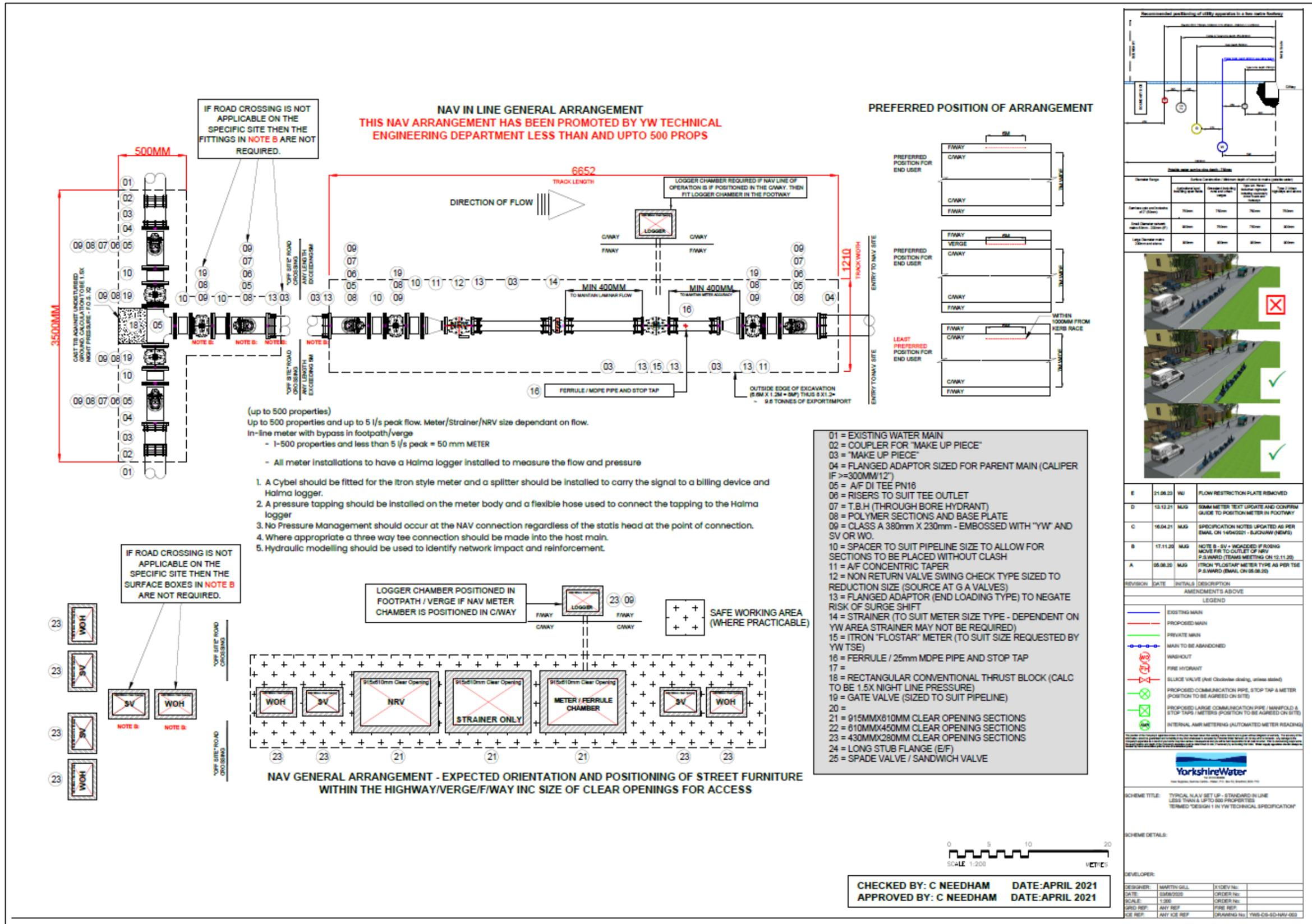
Figure 71: Standard Drawing (NM.001a) NAV General Arrangement (small)
