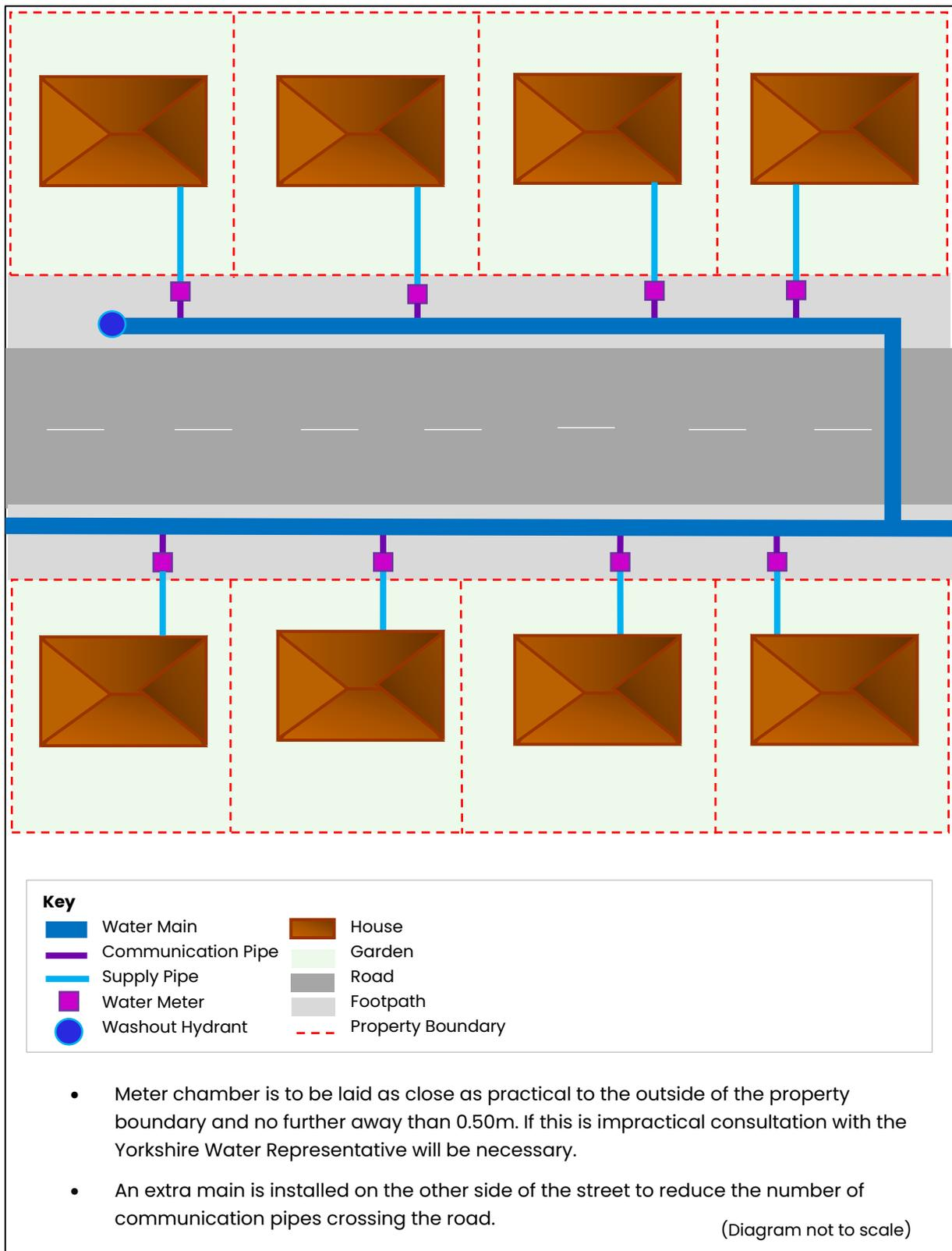
**Figure 29: Standard Drawing (SP.006) Routing and Positioning of Service Pipes – Dual Main**
