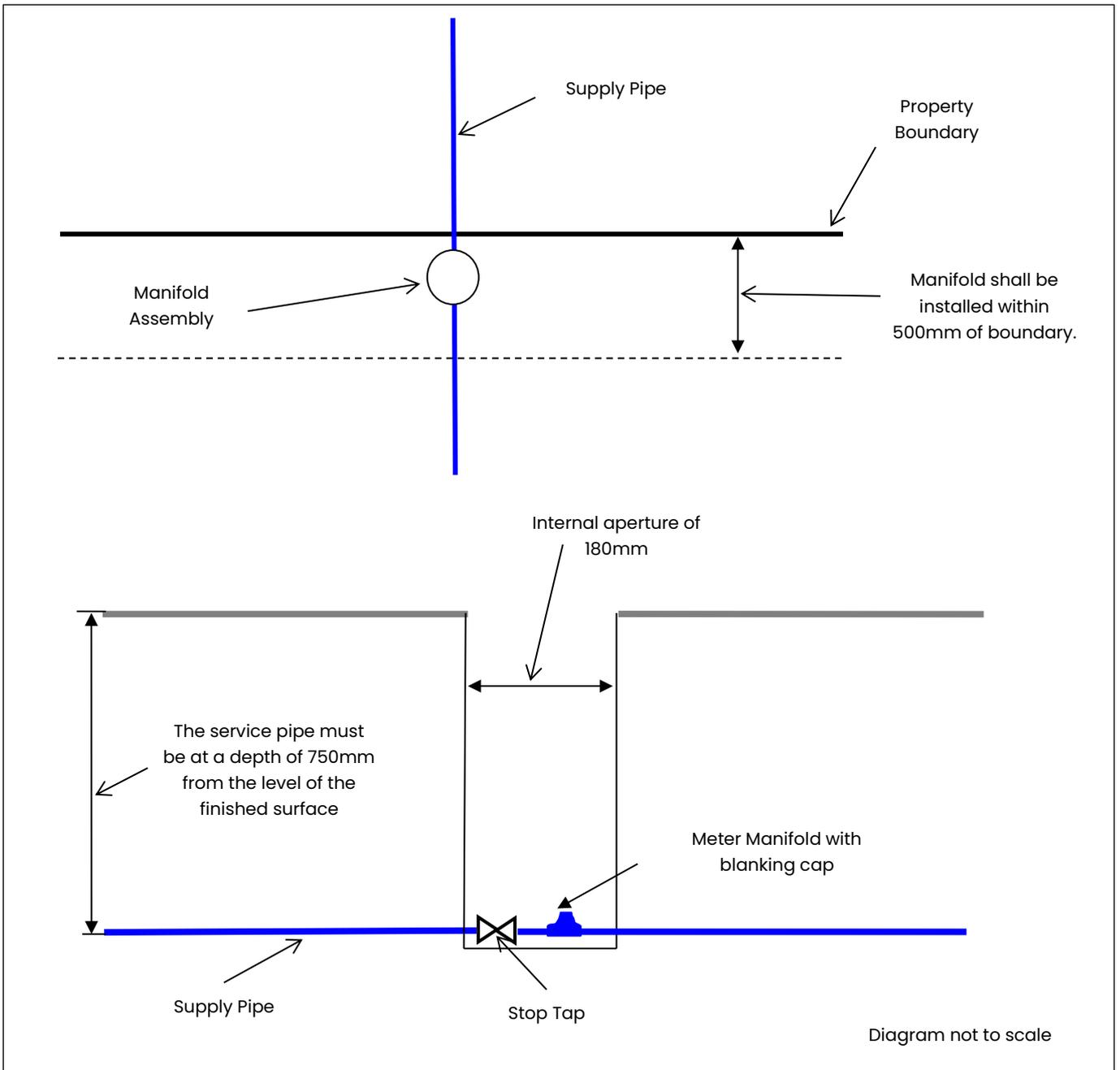
**Figure 53: Standard Drawing (HM.003) MSM Assembly including Meter**
