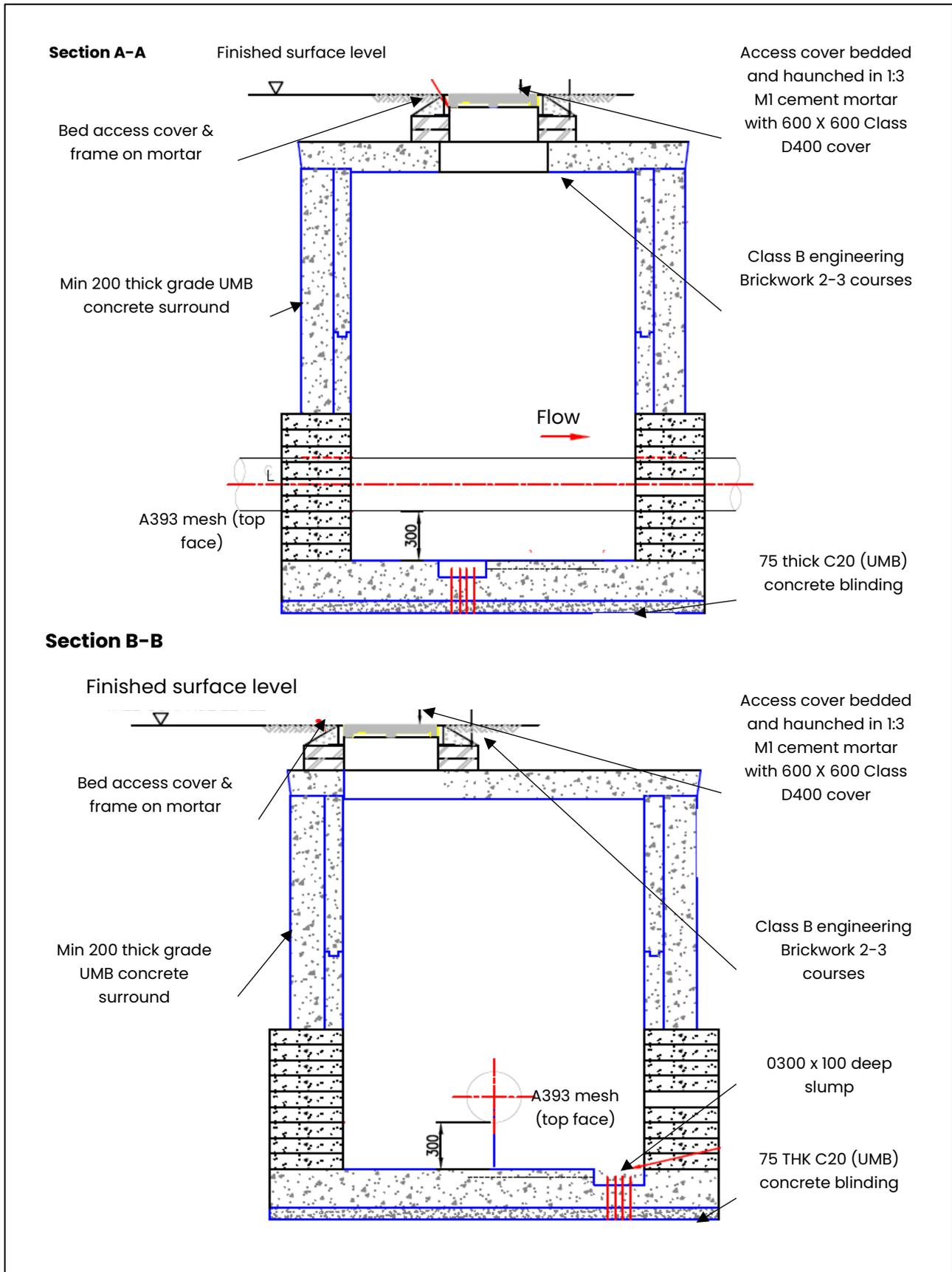
**Figure 50: Standard Drawing (CH.005) Install Chamber around Main**
