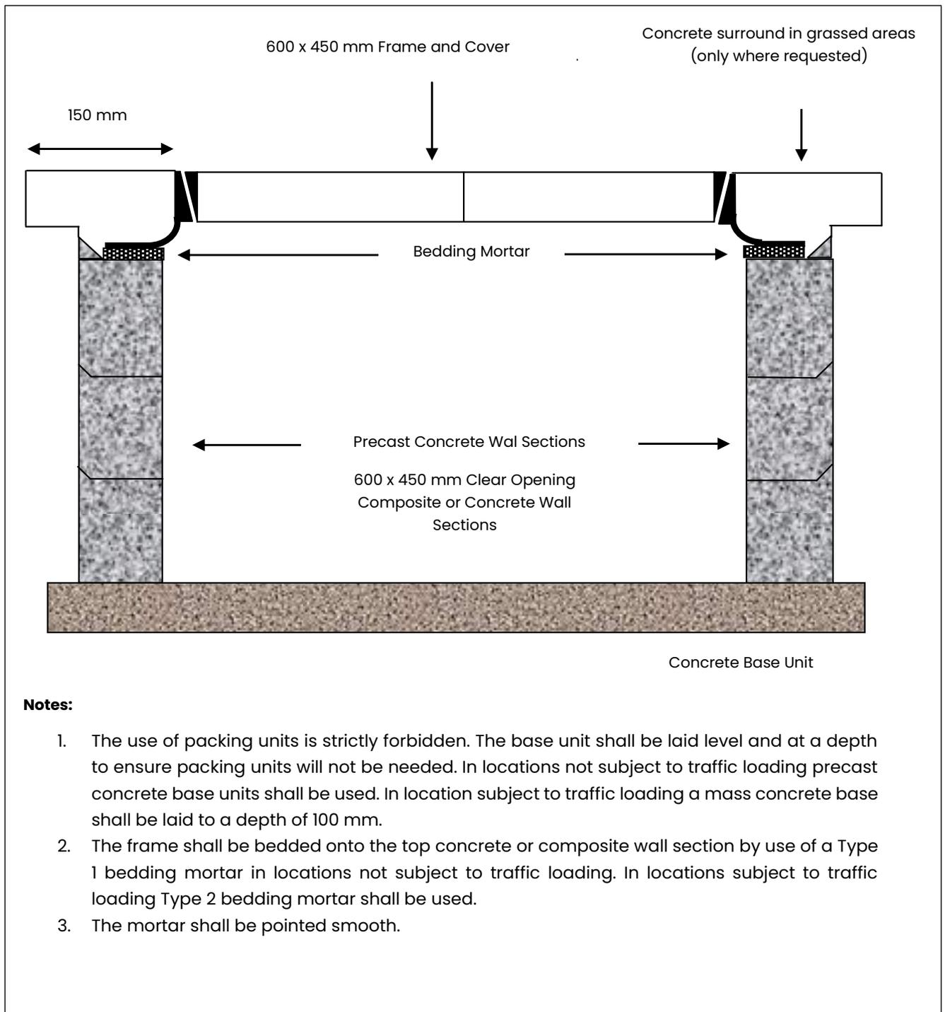
**Figure 48: Standard Drawing (CH.003) Chamber with a 600 x 450 mm Frame and Cover**
