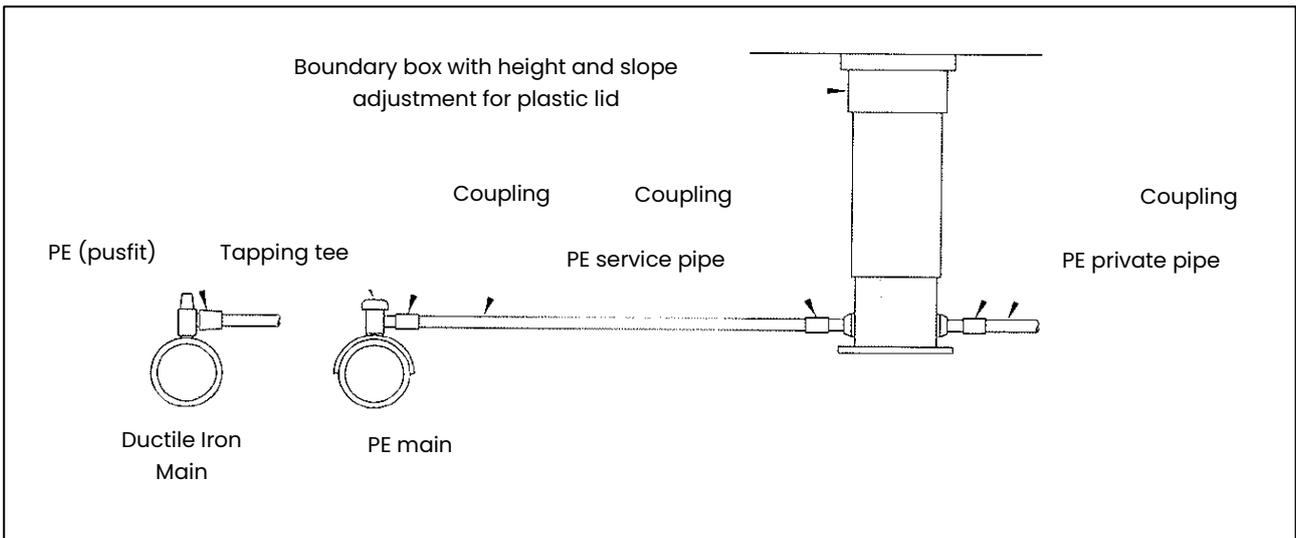
**Figure 24: Standard Drawing (SP.001) Communication Pipe Connection**
