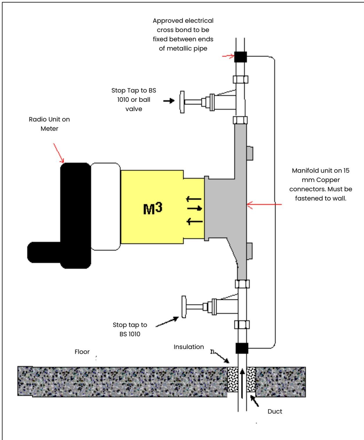
**Figure 54: Standard Drawing (HM.004) Fitting Single Manifold**
