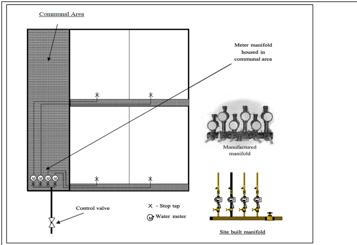
**Figure 64: Standard Drawing (HM.014) Multi Occupancy Building - Internal meters in communal area with individual supplies**
