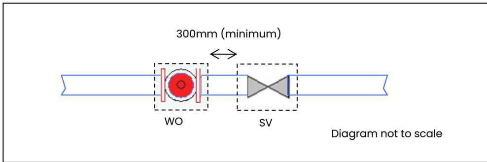
**Figure 43: Standard Drawing (XO.001) Valve and Washout Arrangement**
