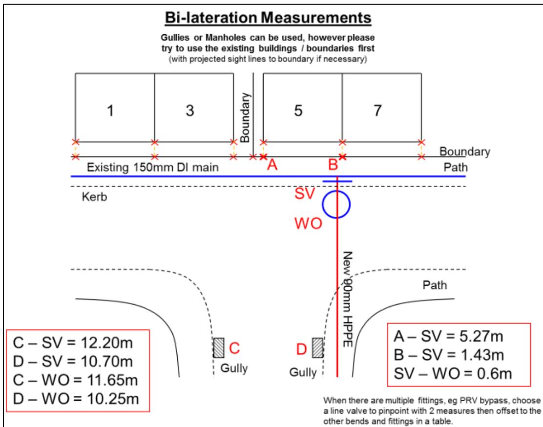
**Figure 18: Example 'As Laid' Drawing – Bi-Lateration Measurements**
