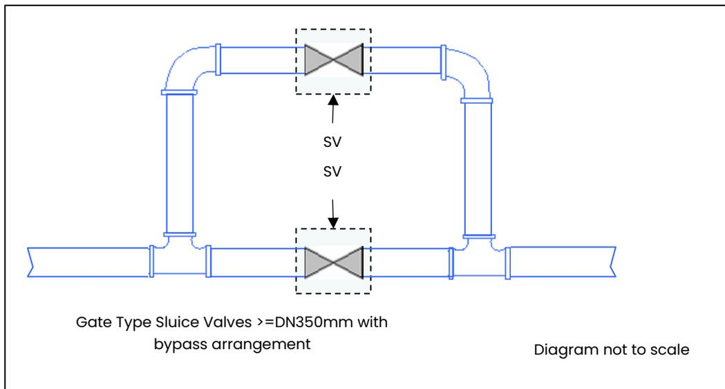
**Figure 39: Standard Drawing (SV.005) Sluice Valve with Bypass**
