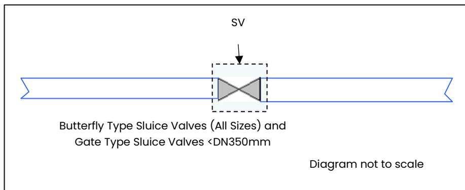
**Figure 38: Standard Drawing (SV.004) Inline Sluice Valve**
