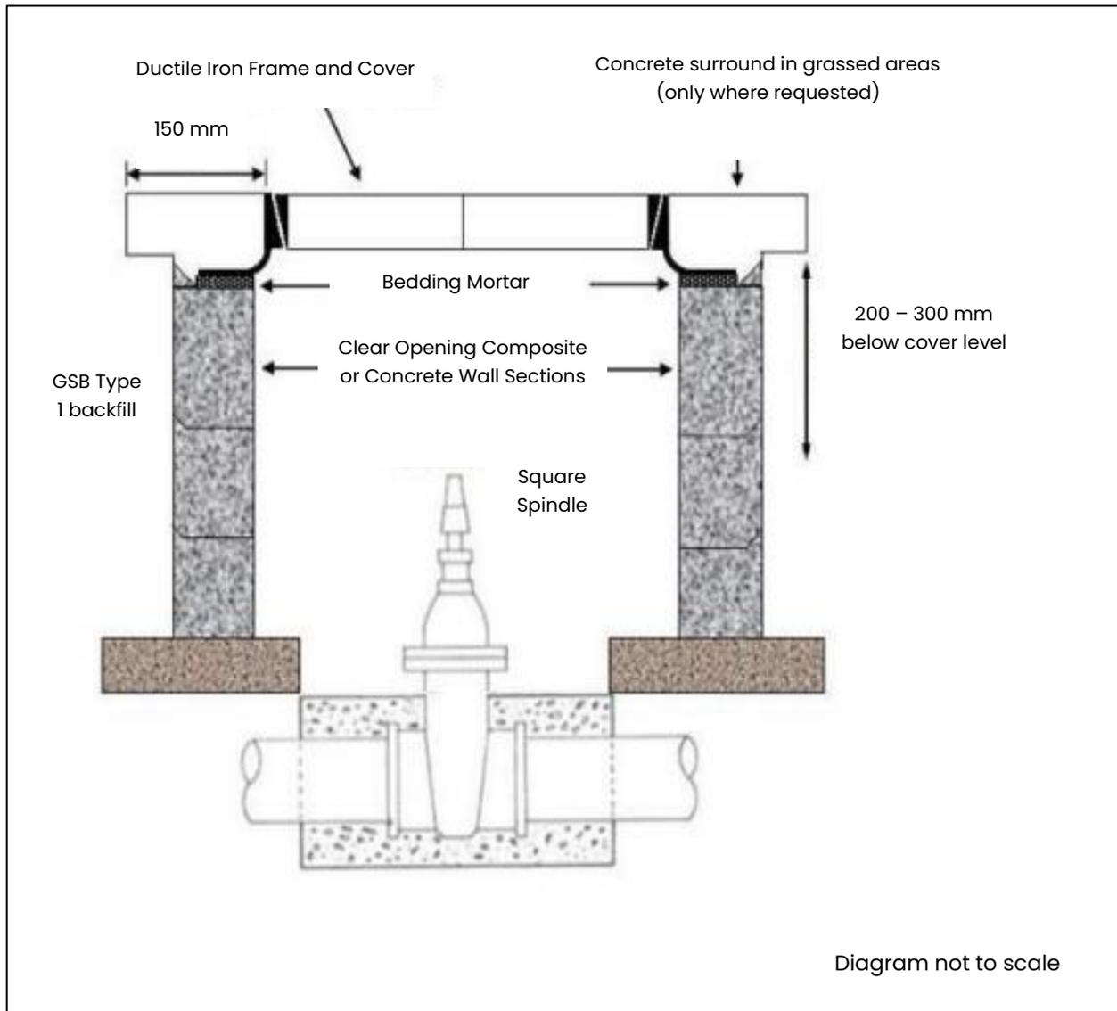
**Figure 37: Standard Drawing (SV.002) Valve within Chamber**
