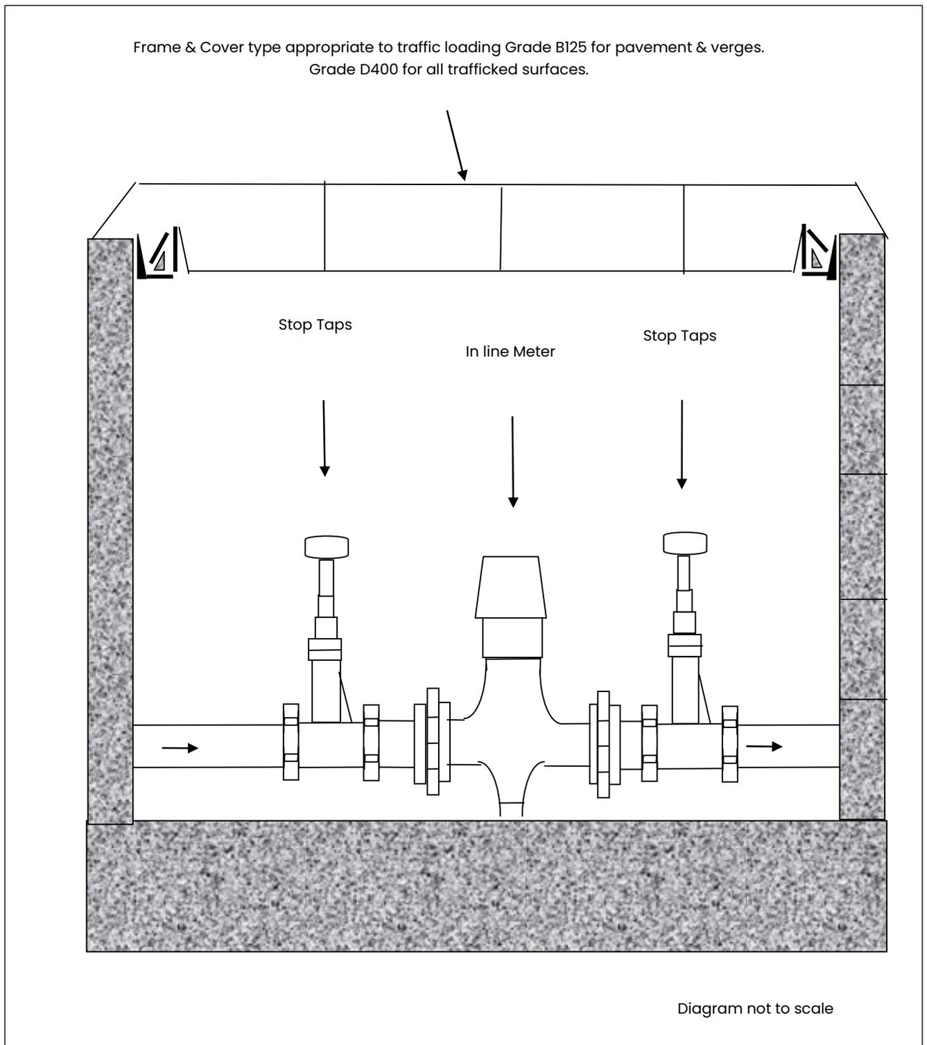
**Figure 61: Standard Drawing (HM.011) External In-Line 20 – 39 mm Meter Installation in a Chamber**
