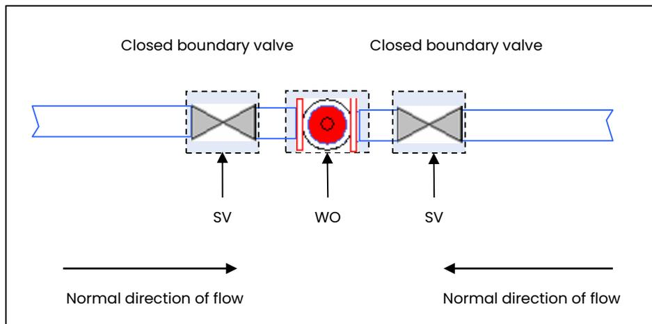
**Figure 45: Standard Drawing (XO.003) XOX Valve-Hydrant-Valve Arrangement**
