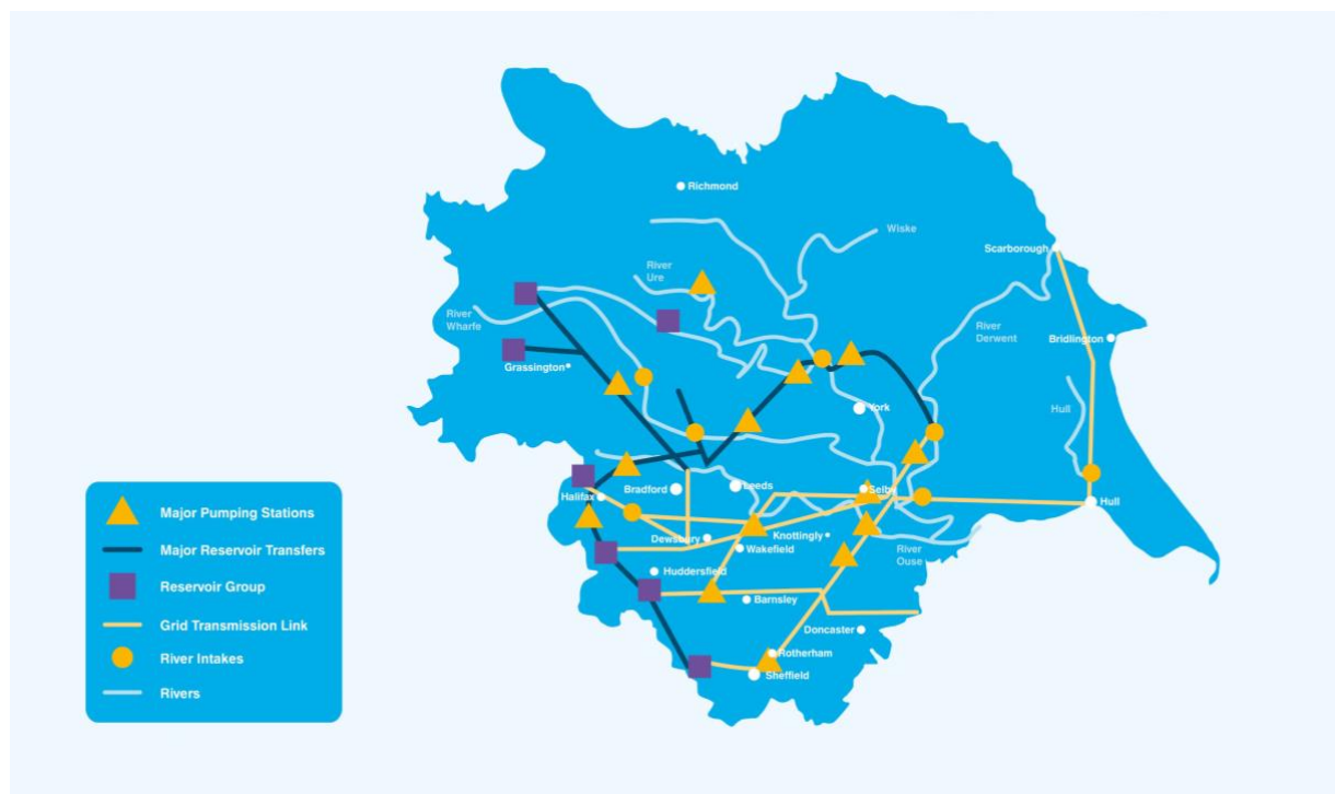
Figure 3.1: Overview of Grid system
