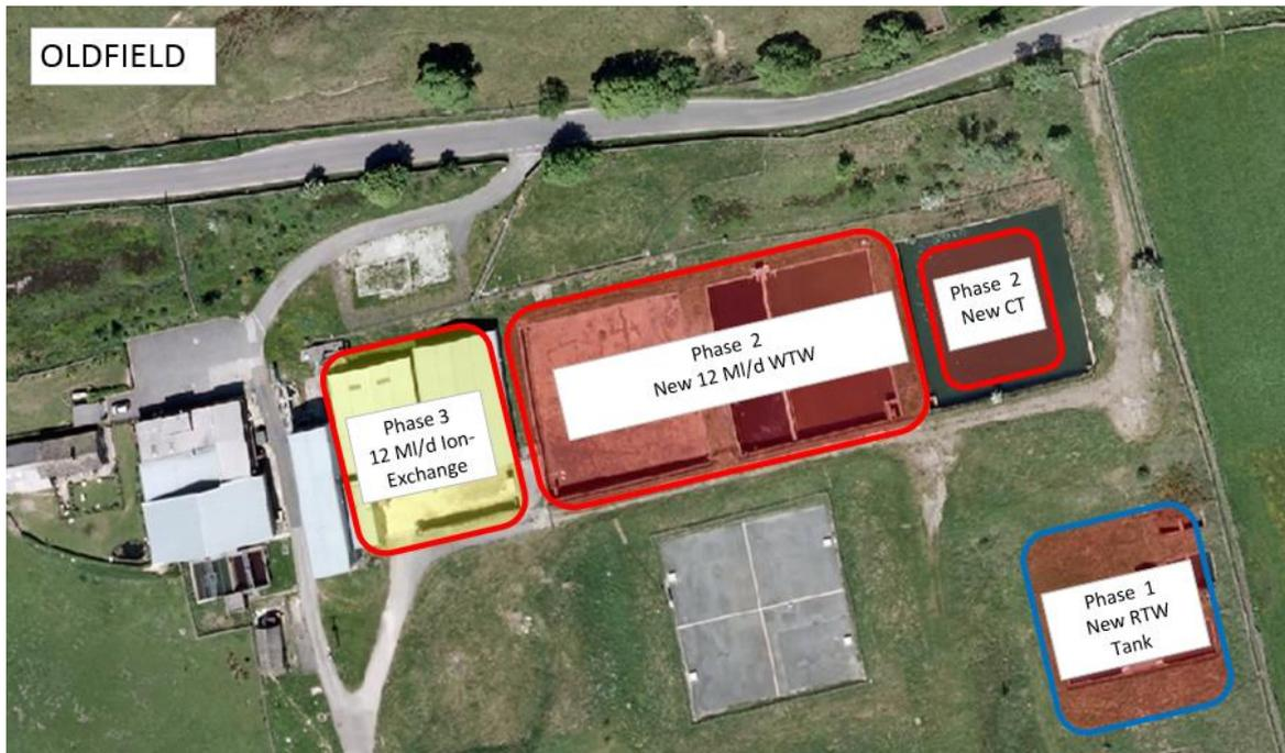
Figure. 17: Proposed location of new or relocated process units.
