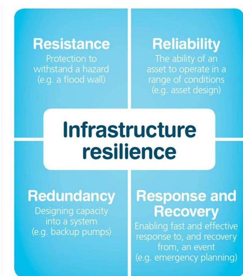
Figure. 9: The components of infrastructure resilience - In building resilience, the contribution made by each of these four components needs to be considered.
