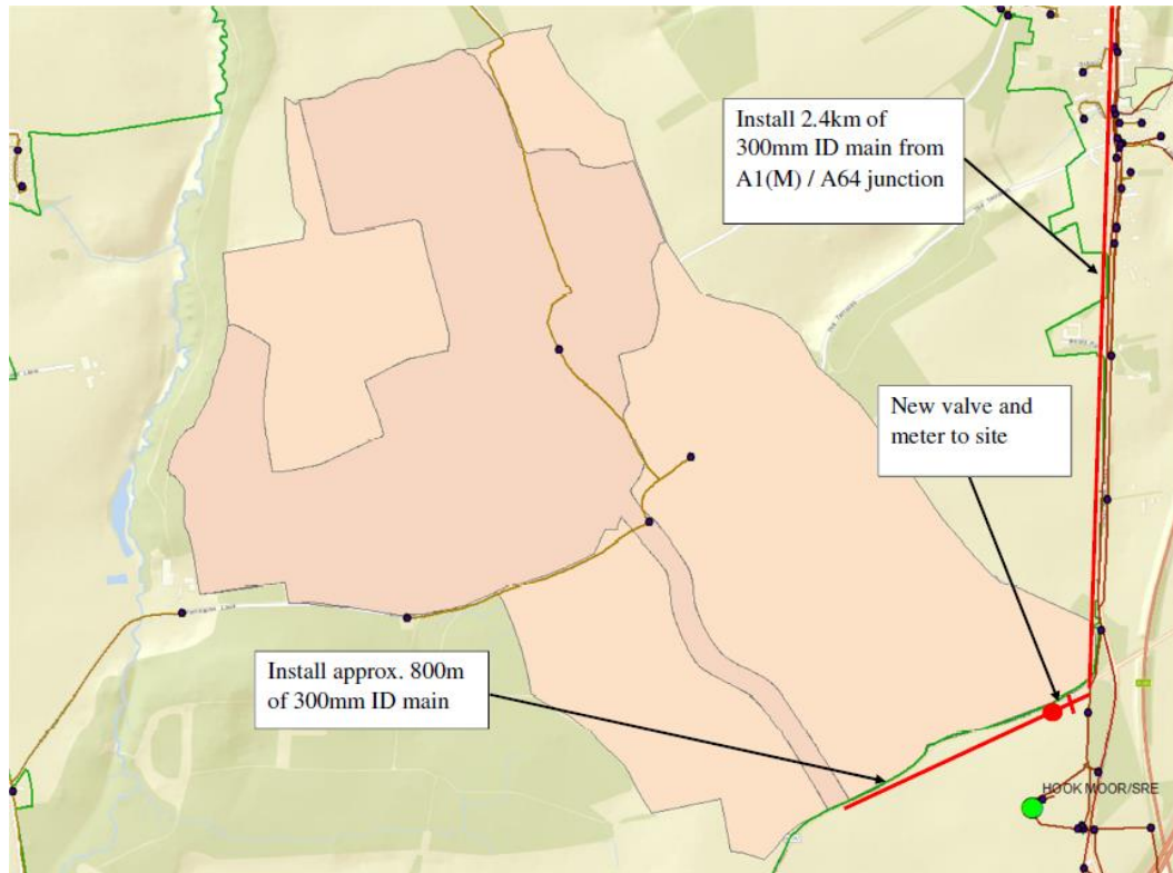
Figure 12: Water supply connection to proposed Parlington site
