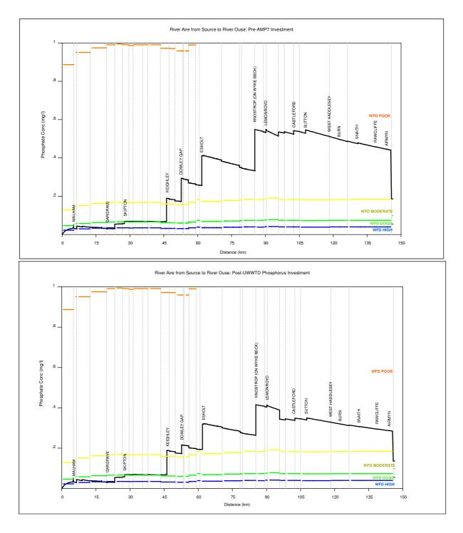
Figure 7.2: Comparison of phosphorous concentrations in the River Aire pre- and post- UWWTD investment
