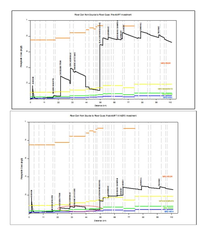
**Figure 7.10 : River** comparison of phosphorous concentrations pre- and post- WFD and UWWTD investment
