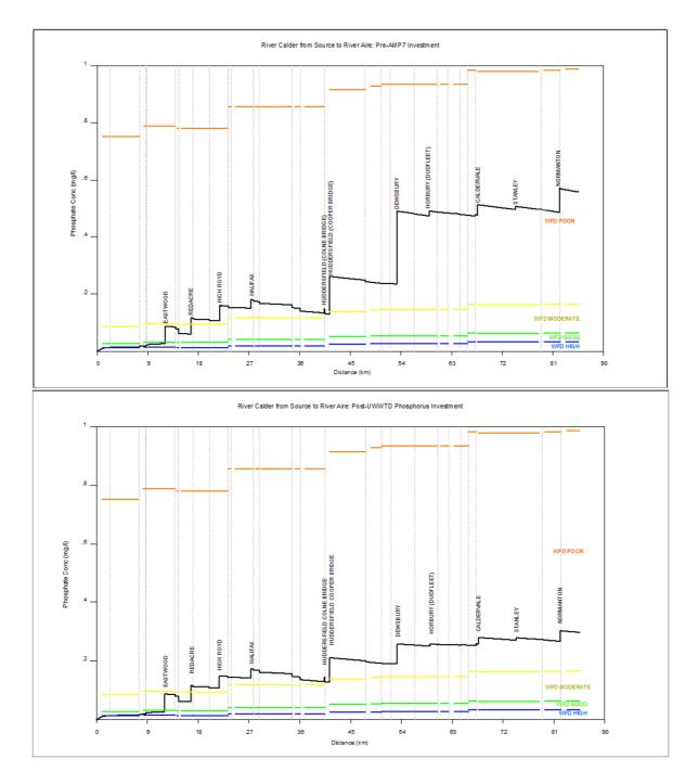
Figure 7.3 : Comparison of phosphorous concentrations in the River Calder pre- and post- UWWTD investment
