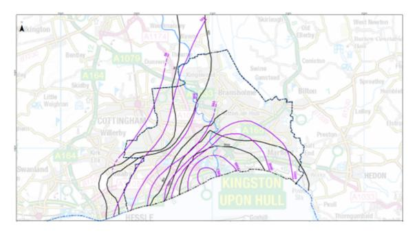
Figure 6.1 isocholors showing current extent of saline intrusion purple lines and extent in 1967 as black lines.
