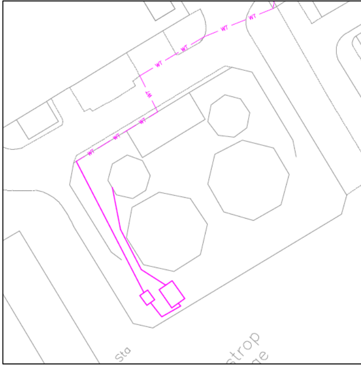
Figure 5 - Indicative layout of the pipework and kiosks for Option 1 (shown in proportion to existing infrastructure)
