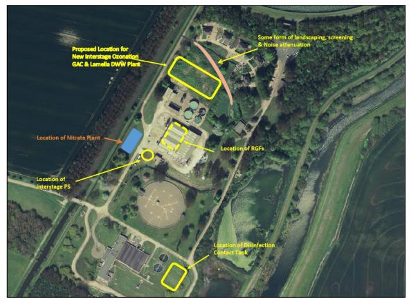
Figure. 48: Proposed location of new or refurbished processes
