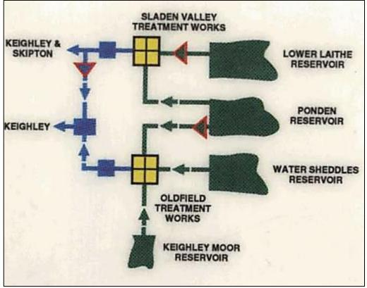
Figure. 16: Oldfield WTW and Sladen Valley WTW raw water supply system.
