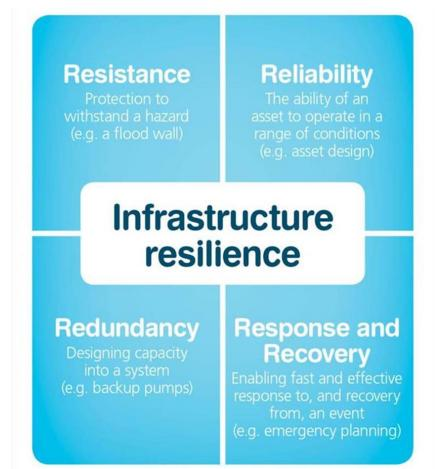
Figure. 9: The components of infrastructure resilience - In building resilience, the contribution made by each of these four components needs to be considered.
