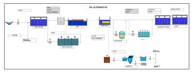
Figure. 50: Process schematic – Alternative solution.
