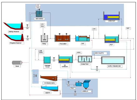
Figure. 29: Proposed solution process schematic.
