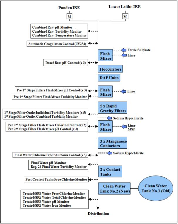
Figure. 25: Process schematic for Sladen Valley WTW.
