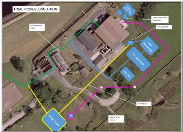
Figure. 36: Embsay WTW: Location of proposed new process units (in blue).
