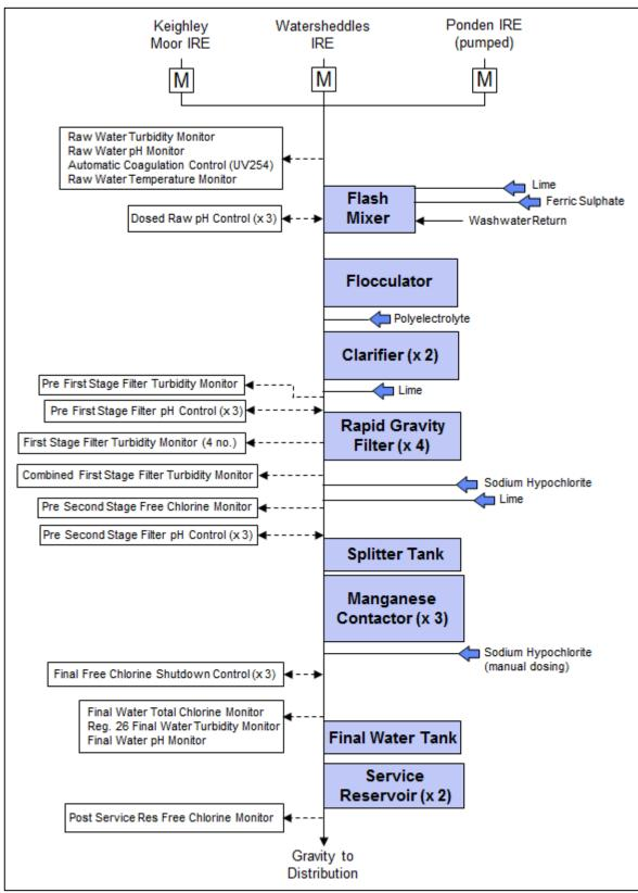
Figure. 17: Process schematic for Oldfield WTW.
