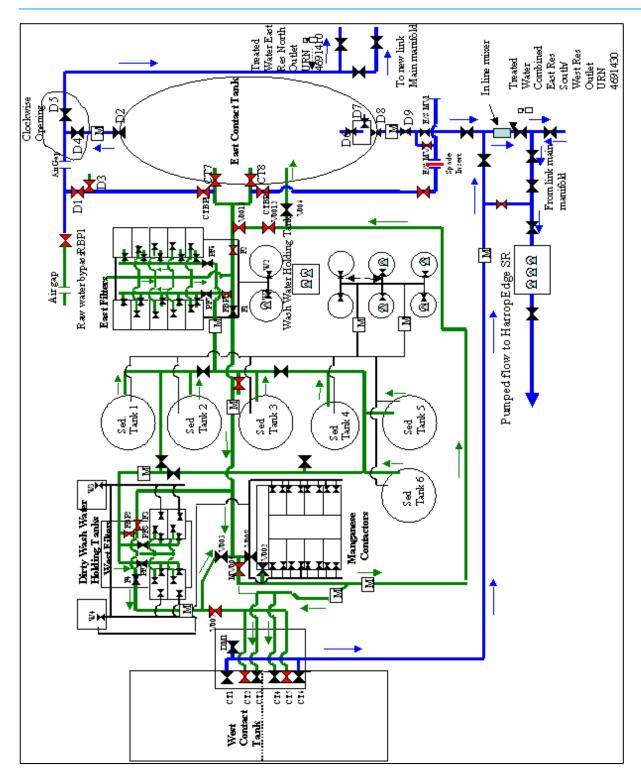
Figure. 1: Site schematic for Chellow Heights WTW.
