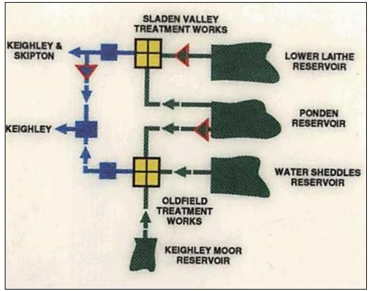
Figure. 24: Oldfield WTW and Sladen Valley WTW raw water supply system.
