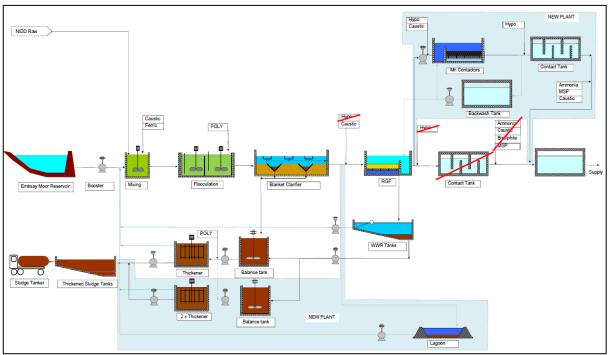
Figure. 37: Proposed solution process schematic.
