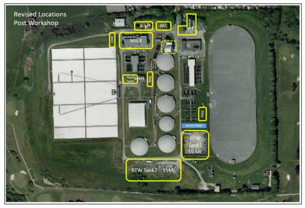
Figure. 12: Proposed location of new or relocated process units – solid lines / replaced process units – dotted line.
