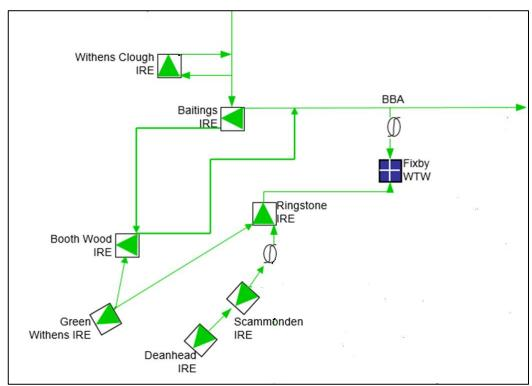
Figure. 26: Fixby raw water supply schematic.
