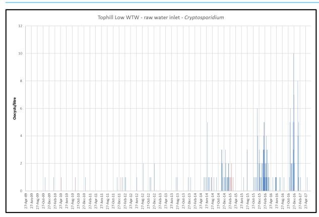
Figure. 45: showing trend in Cryptosporidium oocysts at WTW inlet.
