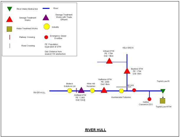
Figure. 28: Flow diagram illustrating water quality risks to River Hull abstraction point.
