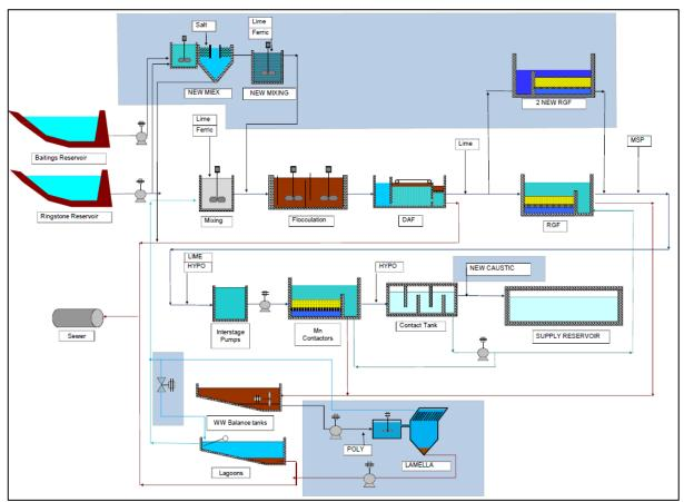
Figure. 31: Alternative solution - Process schematic.
