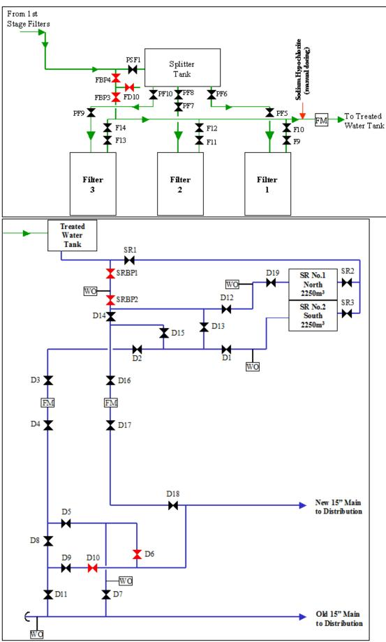
Figure. 15: Site schematic for Oldfield WTW.
