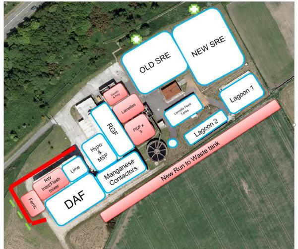
Figure. 28: Proposed location of new or relocated process units – red lines / existing process units – blue line.
