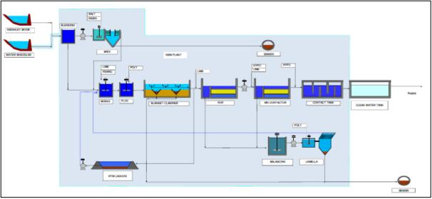
Figure. 18: Proposed solution process schematic.
