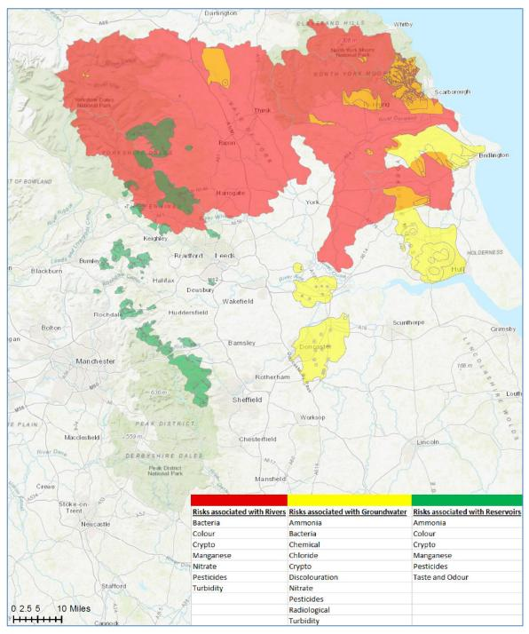
Figure. 9: An overview of the hazards arising in the catchments.
