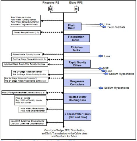
Figure. 13: Process Schematic for Fixby WTW.
