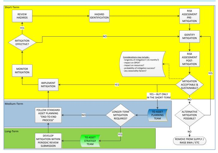
Figure. 3: Process for development of measures following hazard identification.
