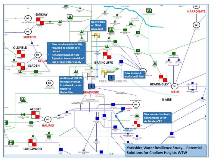
Figure. 43: Chellow Water Supply System: Overview of potential interventions to improve system resilience.
