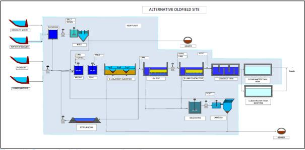
Figure. 20: Proposed solution - process schematic.
