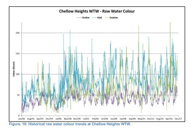
In addition, the site uses aluminium sulphate as coagulant which is less effective at the removal of DOC than ferric sulphate. Trials using ferric sulphate as coagulant were unsuccessful due to the higher alkalinity of the other raw water streams in the blend at Chellow WTW. This results in extremely high acid doses to pH correct the dosed-water to the optimal value for organics removal, along with producing very high sludge volumes.
