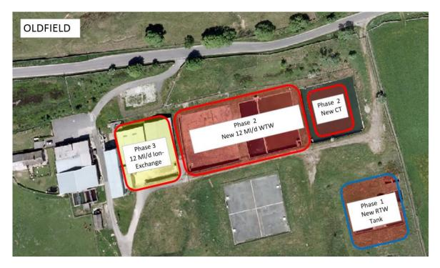
Figure. 17: Proposed location of new or relocated process units.
