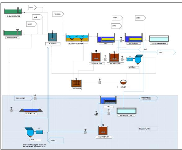
Figure. 15: Proposed solution process schematic.
