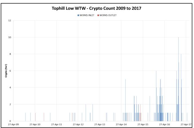
Figure. 32: Chart displaying crypto detected at Tophill Low WTW inlet and outlet from 2009 to 2017.
