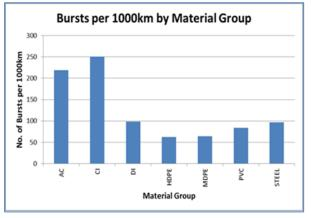
Figure. 32: Network maintenance data, comparing burst rates with different materials of construction.
