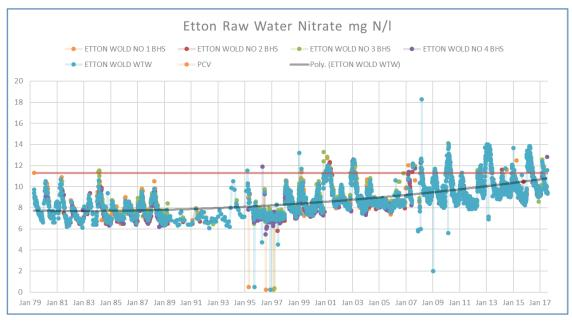
Figure. 22: Groundwater nitrate concentration at Etton abstraction from 1979 to 2017.
